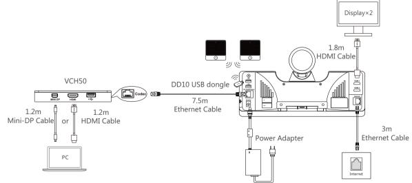
$\bigcirc$  The CPW90 wireless microphones and DD10 USB dongle are automatically paired from the factory.
