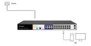
Step2、Manually changed the computer IP address to 192.168.254.X (X is  $2 \sim 254$ ), subnet mask is 255.255.255.0
